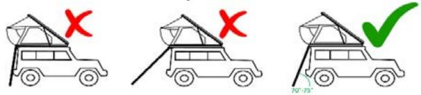
The ladder may need to be adjusted to achieve the correct angle depending on the height of your setup. If shortening is required, the adjustment must be done from the top.
