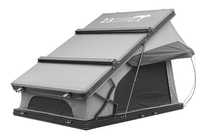
**Note:** The roof bars supplied with the Kabari Series Hardshell Roof Top Tent are not designed to carry significant loads. A maximum of 45 lbs can be carried on top of the Kabari Series Hardshell Roof Top Tent providing this weight is spread evenly amongst the 2 bars. When adding additional weight to the top of the tent, consideration must be given to the overall weight rating capacity of your vehicle's roof and roof rack.
