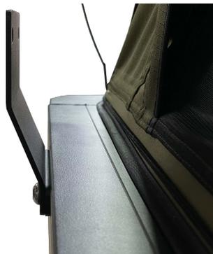
3. Using (2) M8 bolts, place the raised window fly plate into the channel nuts ensuring the backing plate is attached on inside.
