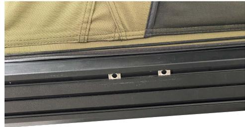
2. Once removed, leave the existing channel nuts in the original spot.
