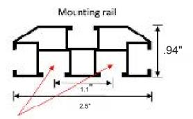
Slide mounting bolt in to either channel.
