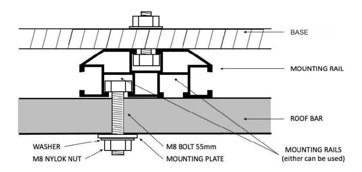
**Note:** It is recommended the rear of the tent is flush with the back of the vehicle to allow correct ladder angle. Place a mounting plate under the roof bar whilst locating the bolts, insert washer and hand tighten lock nut. Repeat for all 4 corners. Double check the tent's position as desired and tighten all nuts securely with 13mm wrench. Insert end caps into the ends of the mounting rails, this may require light taps from a hammer.
