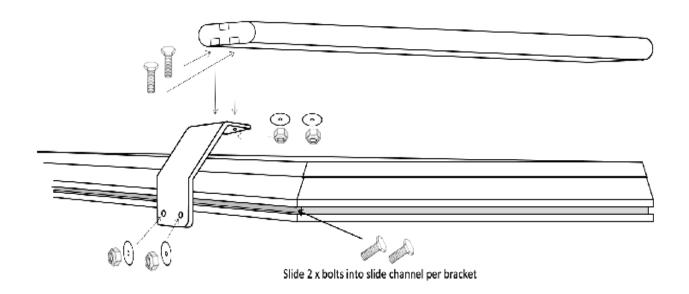
**Note:** A maximum of 44 lbs can be carried on top of the KABARI 2.0 providing this weight is spread evenly amongst all three bars. Load weights greater than 40 lbs will void any warranty.
