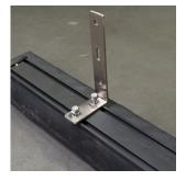
Once the brackets are in the desired position, tighten the nuts.
