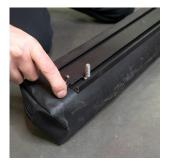
Attach L-Brackets to bolts and loosely secure nuts. Be sure not to tighten as you may need to adjust the position of the brackets.
