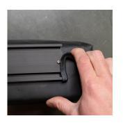
Insert 2 or 3 awning track bolts into the top channel and repeat on bottom channel. This depends on how many L-Brackets you will be using.
