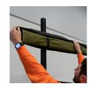
Undo and release the awning using the Velcro straps. Be careful to hold the awning as it will fall when the straps are released.
