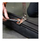
Using the mounting bolts, secure awning to rack.
